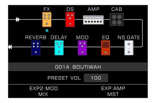
Note:1 .All the modules will display based on the default CHAIN sequence when they' re turned on, as for the CHAIN sequence changed by the users, you need to press SAVE and then they can be saved in the preset tones.
