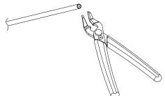
Cut the cable to the desired length using the included cable cutter.
